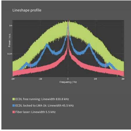
The LWA-1k-1550 featuring an improved resolution enables the analyzation of laser with very narrow linewidths down to 2 kHz. The analyzer unit automatically generates an output signal that is evaluated by the digitizer unit, connected to a PC via USB. An intuitively usable software interface performing the analysis provides the frequency noise related plots and values, such as the frequency noise spectrum and the lineshape spectrum together with the results of intrinsic and combined linewidth.
